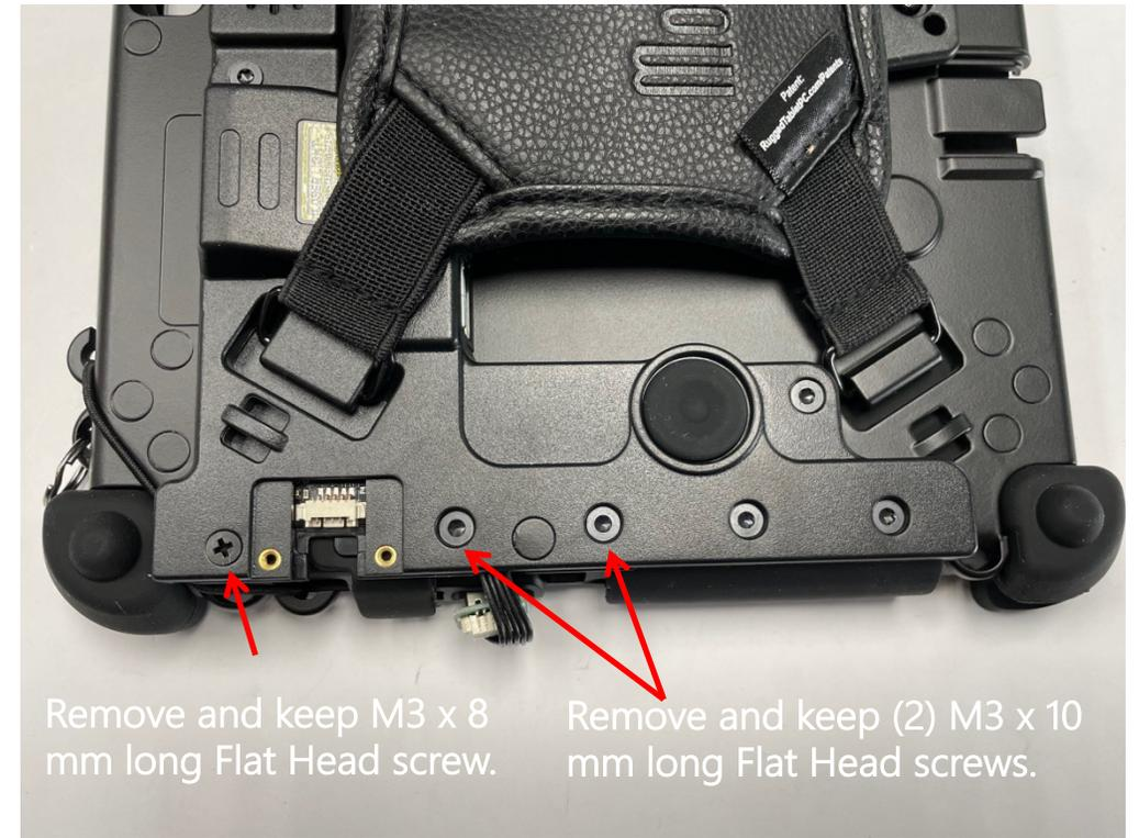
Remove and keep M3 x 8 mm long Flat Head screw.
