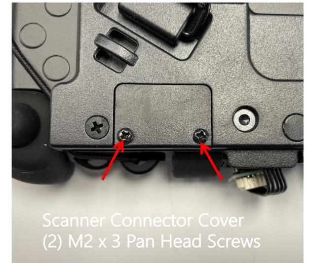
6 - Install the Scanner Connector Cover using (2) M2 x 3 Pan Head screws.
