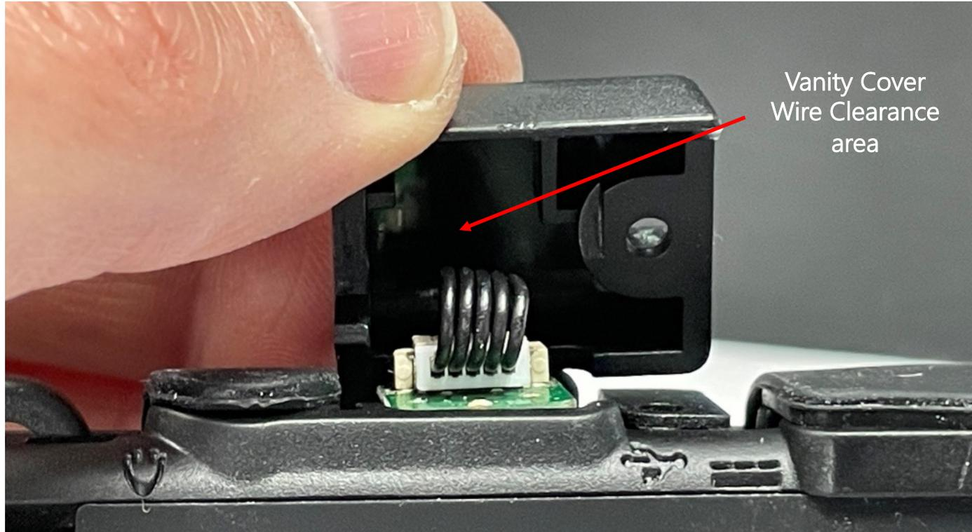
9 - Install Vanity Cover over USB Type C PCB. Ensure wires are aligned in Vanity Cover clearance area so that wires are not pinched.
