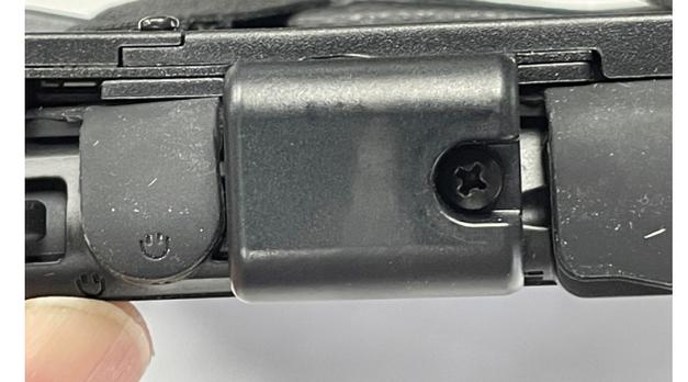
10 - Install the M3 x 5 Pan Head screw.
