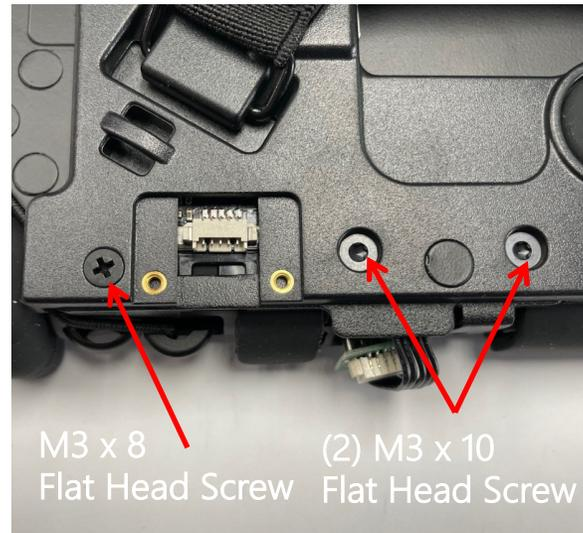
5 - Re-install the M3 x 8 and (2) M3 x 10 Flat Head screws.
