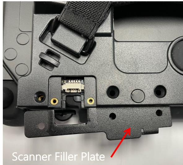
4 - Install the Scanner Filler Plate.
